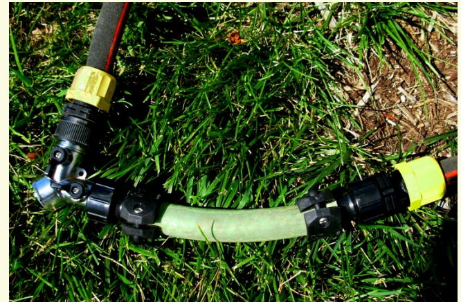
"Gender bender" to improve uniformity of water flow
