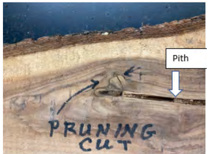
Figure 3. Note how close to the pith this pruning cut was made. The limb was pruned early so wood accumulated to compartmentalize the wound. Rapid growth of the tree effectively compartmentalized the wound by covering it with wood. Note, there is no perceptible bump in the log. Clear wood is covering the wound.
