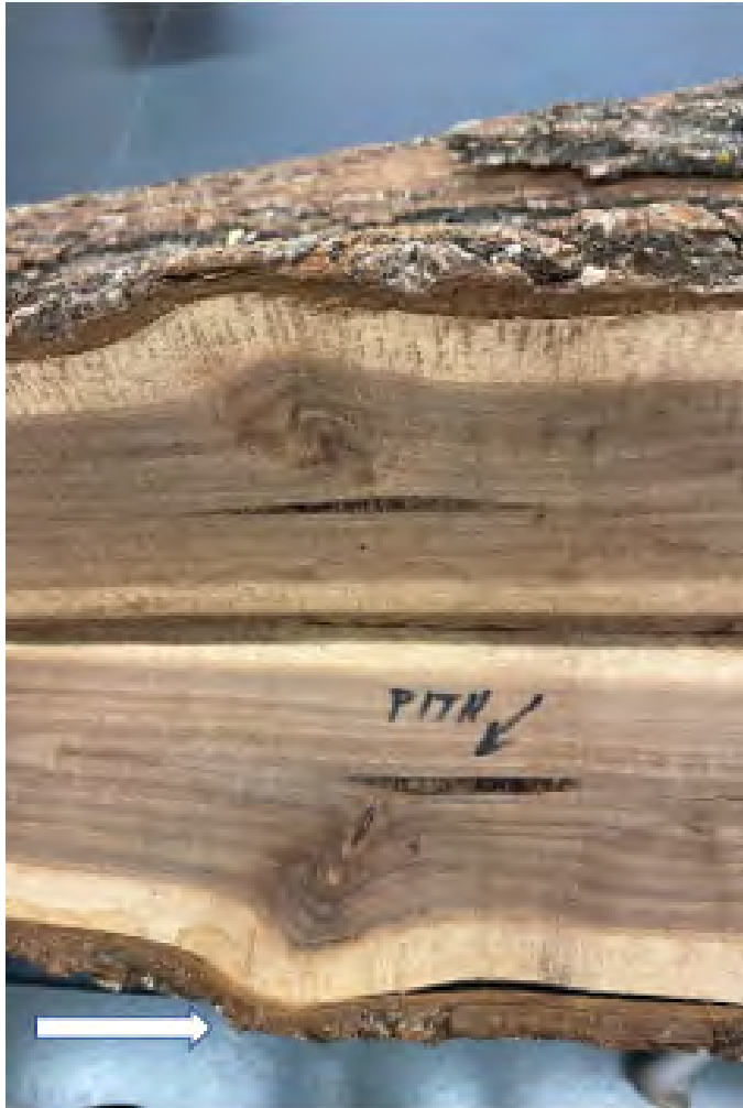
Figure 2. The log was sawed to reveal the inside or heart center of the log. Arrow pointing to the bump where wood has formed around the knot from a pruned limb. Note, the limb originates at the pith; it's the biological center of the tree. The limb as living when pruned but wood rapidly compartmentalized the wound so little decay is present
