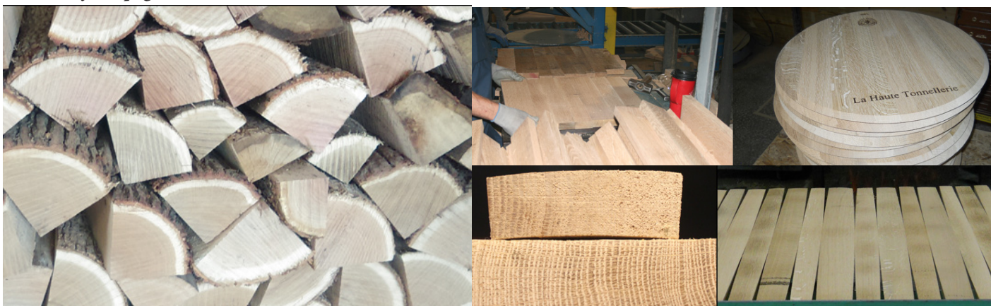
Quarter-sawn stave bolts (left) are sawed into flat stave blanks and trimmed of defects. The blanks either go into header blanks for the top and bottom of the barrel (top right) or into stave blanks (lower right). The cross-section of each stave is a trapezoid and the wider in the middle to give the barrel its barrel shape.
