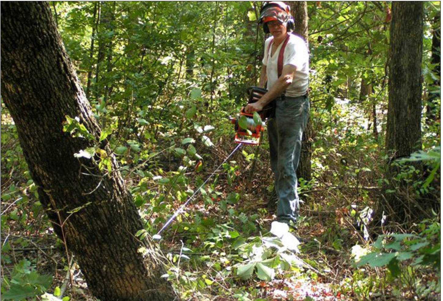
A chainsaw-powered winch is a safe, effective way to bring down a hung tree. Directional felling is so accurate I had to stage this photo, since I rarely have this problem.
