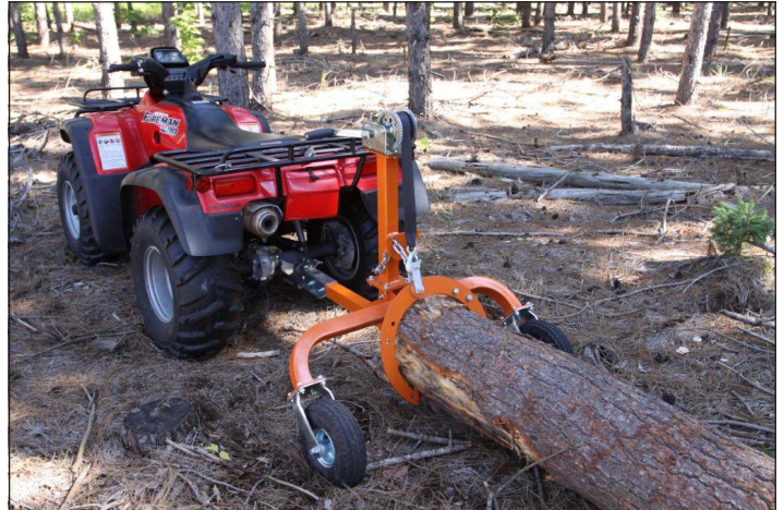
A four-wheel drive ATV can skid firewood and small sawlogs, with the assistance of a log arch. Filling the tires with fluid gives the ATV more traction and stability. The arch bears some of the weight of the log, and lifts the front of the log off the ground.
