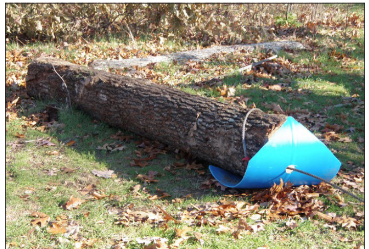
The author's home-made skidding sled for winching logs out of tight places. The sled was made from a plastic 55 gallon barrel, and keeps the end of the log from plowing into the ground and hanging up on stumps.
