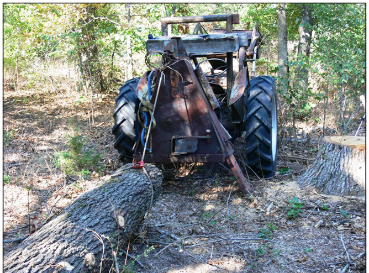
Even an old 8N Ford tractor can be an effective logging machine when fitted with a PTO-powered winch. It isn't fast, but it is inexpensive, and it gets the job done.
