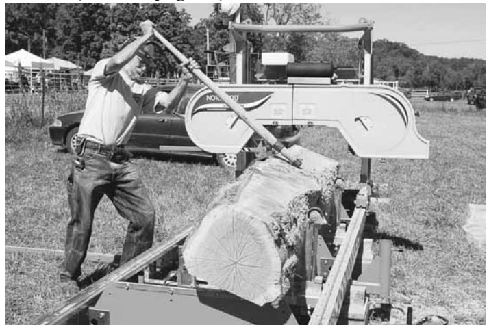
With no hydraulic assist, Boyt wrestles a post oak log around for the next cut. These logs were salvaged from the May 22, 2011 Joplin tornado.
