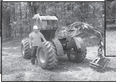
First-generation, small-scale skidder for transporting small-diameter trees to the landing.
