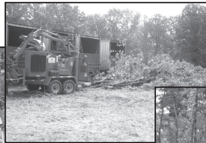
Once to the landing, the biomass is chipped and blown into 25-ton chip vans for transport.
