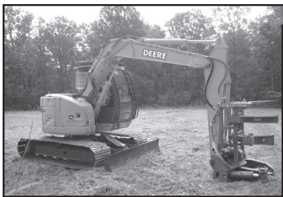
A hydraulic shear head capable of accumulating several small-diameter trees is mounted to a small track-ho for maneuverability.
